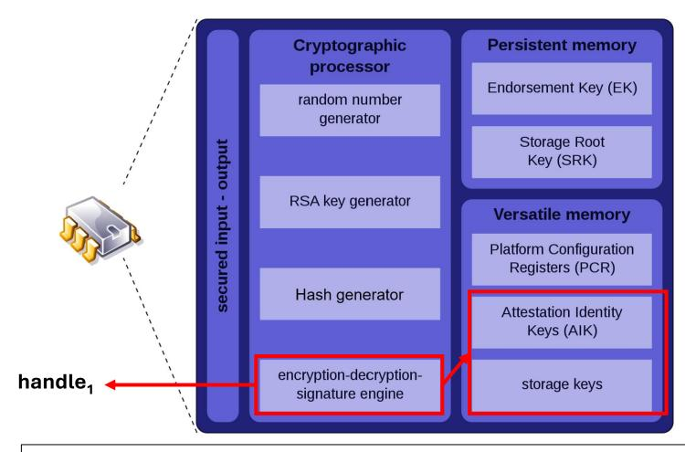
Once key is loaded, the handle can be given as input to other TPM commands
