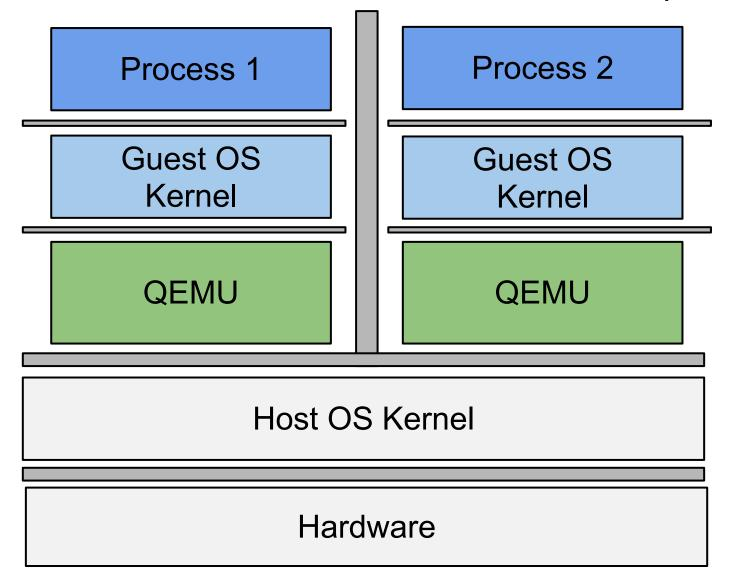
**Definition:** compartmentalization of a program P is (1) a policy to separate P into two or more protection domains (called compartments), and (2) the enforcement of this policy at runtime
